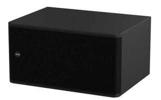
The Venu 215 V2 is a double 15" reflex-loaded low frequency enclosure, providing a frequency response of 38 Hz - 160 Hz  $\pm$ 3 dB and efficiency of 101 dB. Features include tough 15" high excursion transducers with 3" voice coils and a durable enclosure made entirely from 18 mm multi-laminate birch plywood.
