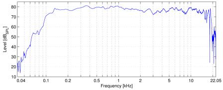
Frequency response (Anechoic measurement)
