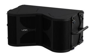
Specially designed to extend the low frequency range of the Arcline line array, the Arcline 212 features two 12" 900 W low frequency drivers. This makes it possible to extend the frequency response range to as low as 50 Hz, while also reaching up to 200 Hz.
