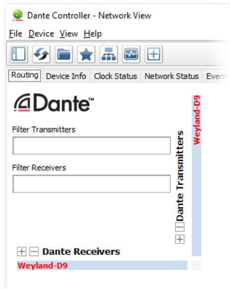
Figure 6 - Dante Controller showing device in failsafe mode
