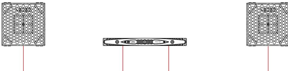
Figure 5.3: 2 x Nexus X: 4 Ω per channel / 1 amplifier
